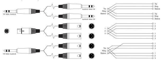
Headphone Separator Note: for every doubling of headphones the load impedance is halved. Do not go below 32 Ohms.
